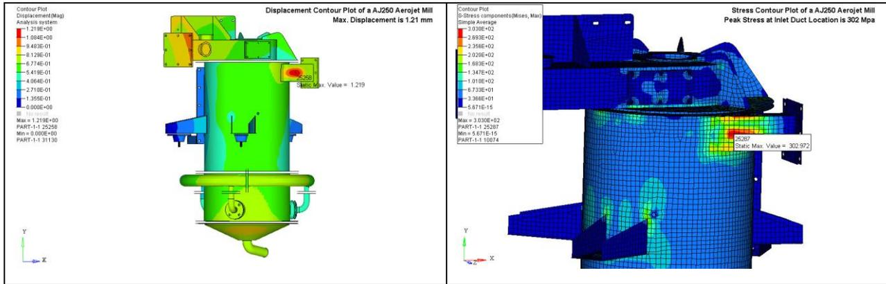
Figure 4: Displacement and Stress Contour Plots of a Dynamic Analysis of AJ250 Aerojet Mill Assembly
