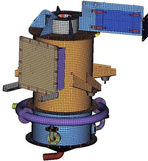
Figure 2: FE Model of an AJ250 Aerojet Mill
