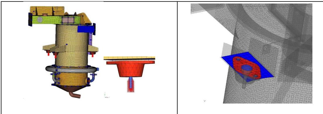
Figure 3: Boundary Conditions and Contact pairs
